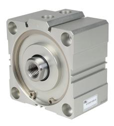
NITRA pneumatic cylinder, compact extruded, 100mm bore, 32mm rod diameter, 10mm stroke, double acting, magnetic piston, tapped end caps mount.
