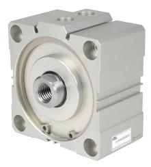
NITRA pneumatic cylinder, compact extruded, 100mm bore, 32mm rod diameter, 5mm stroke, double acting, magnetic piston, tapped end caps mount.
