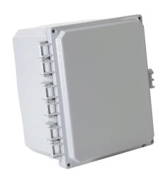
Integra Premium series enclosure, NEMA 1/2/3/3R/3S/4/4X/12/13, 10 x 8 x 6in (HxWxD), wall mount, polycarbonate, light gray, gloss finish, single-door, glass-filled nylon quick-release latch, padlock hasp and staple.
