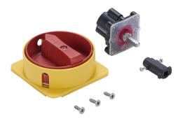
Merz rotary handle, round, red/yellow, external front mount, 2-position, lockable in OFF only, NEMA 4/4X. For use with Merz ML2 & ML3 switch bodies in DIN rail applications with hinged doors. Shaft adapter and mounting screws included.
