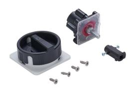
Merz rotary handle, round, black/gray, external front mount, 2-position, lockable in OFF only, NEMA 4/4X. For use with Merz ML1 switch bodies in DIN rail applications with hinged doors. Shaft adapter and mounting screws included.
