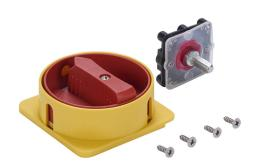
Merz rotary handle, round, red/yellow, external front mount, 2-position, lockable in OFF only, NEMA 4/4X. For use with Merz ML2 & ML3 switch bodies in DIN rail applications with non-hinged doors. Shaft adapter and mounting screws included.
