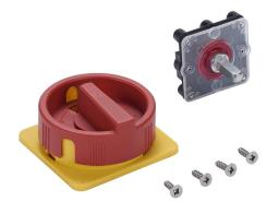
Merz rotary handle, round, red/yellow, external front mount, 2-position, lockable in OFF only, NEMA 4/4X. For use with Merz ML1 switch bodies in DIN rail applications with non-hinged doors. Shaft adapter and mounting screws included.
