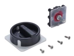
Merz rotary handle, round, black/gray, external front mount, 2-position, lockable in OFF only, NEMA 4/4X. For use with Merz ML1 switch bodies in DIN rail applications with non-hinged doors. Shaft adapter and mounting screws included.
