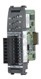
DirectLOGIC DL05/06 pulse combo module, 250 kHz maximum switching frequency, 4 high-speed input point(s), sinking/sourcing, single-ended encoder input(s), 2 high-speed output point(s), sinking/sourcing, single-ended output(s).
