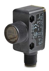
AutomationDirect photoelectric sensor, rectangular, plastic housing, through-beam receiver, right-angle lens, 20m sensing distance, 10-30 VDC operating voltage, dark-on, PNP, 3-wire, 4-pin M12 quick-disconnect.
