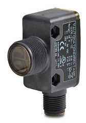
AutomationDirect photoelectric sensor, rectangular, plastic housing, through-beam receiver, right-angle lens, 20m sensing distance, 10-30 VDC operating voltage, dark-on, NPN, 3-wire, 4-pin M12 quick-disconnect.
