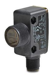
AutomationDirect photoelectric sensor, rectangular, plastic housing, through-beam receiver, right-angle lens, 20m sensing distance, 10-30 VDC operating voltage, light-on, PNP, 3-wire, 4-pin M12 quick-disconnect.
