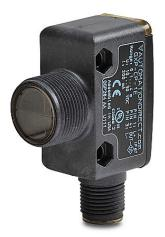
AutomationDirect photoelectric sensor, rectangular, polarized retroreflective, right-angle lens, visible red light emission, 4m sensing distance, dark-on, PNP, 3-wire, 4-pin M12 quick-disconnect.
