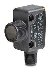
AutomationDirect photoelectric sensor, rectangular, polarized retroreflective, right-angle lens, visible red, 4m sensing distance, dark-on, NPN, 3-wire, 4-pin M12 quick-disconnect.
