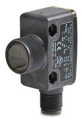
AutomationDirect photoelectric sensor, rectangular, polarized retroreflective, right-angle lens, visible red, 4m sensing distance, light-on, PNP, 3-wire, 4-pin M12 quick-disconnect.
