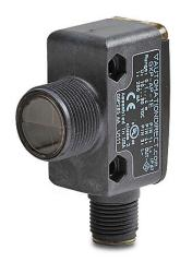
AutomationDirect photoelectric sensor, rectangular, polarized retroreflective, right-angle lens, visible red light emission, 4m sensing distance, light-on, PNP, 3-wire, 4-pin M12 quick-disconnect.
