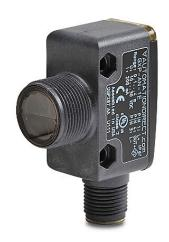
AutomationDirect photoelectric sensor, rectangular, polarized retroreflective, right-angle lens, visible red, 4m sensing distance, light-on, NPN, 3-wire, 4-pin M12 quick-disconnect.
