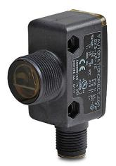
AutomationDirect photoelectric sensor, rectangular, plastic, diffuse with background suppression, right-angle lens, 100mm sensing distance, light-on, PNP, 1 kHz switching frequency, 4-pin M12 quick-disconnect.
