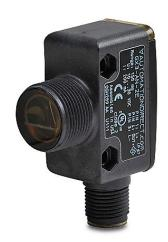
AutomationDirect photoelectric sensor, rectangular, plastic, diffuse with background suppression, right-angle lens, 150mm sensing distance, light-on, NPN, 1 kHz switching frequency, 4-pin M12 quick-disconnect.
