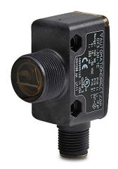
AutomationDirect photoelectric sensor, rectangular, plastic, diffuse with background suppression, right-angle lens, 100mm sensing distance, light-on, NPN, 1 kHz switching frequency, 4-pin M12 quick-disconnect.
