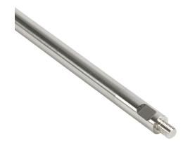
ProSense level sensing probe, 1000mm length, stainless steel. For use with GWR-1600-C and GWR-1600-P guided wave radar level sensors and CLC series conductive level controllers.
