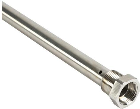
ProSense coaxial tube, 1200mm length, 3/4in male NPT process connection, stainless steel. For use with GWR-1600-C guided wave radar level sensors. (1) centering piece included.
