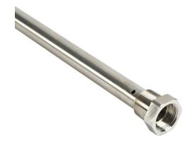
ProSense coaxial tube, 1200mm length, 3/4in male NPT process connection, stainless steel. For use with GWR-1600-C guided wave radar level sensors. (1) centering piece included.
