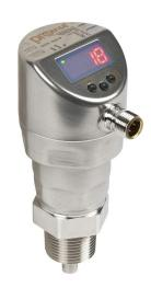
ProSense probe guided wave radar water level sensor, 1570mm maximum sensing range, Output: switch, Output 2: switch or analog, 18-30 VDC operating voltage, 3/4in male NPT process connection.
