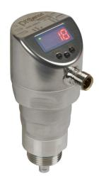
ProSense coaxial guided wave radar water and oil level sensor, 1570mm maximum sensing range, Output: switch, Output 2: switch or analog, 18-30 VDC operating voltage, G3/4 male BSPP process connection.
