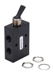
NITRA pneumatic manual valve, 5-port (4-way), 2-position, toggle style actuator, detented, 1/8in female NPT inlet(s), 1/8in female NPT outlet(s), 1/8in female NPT exhaust(s), Cv=0.37, through panel mount.
