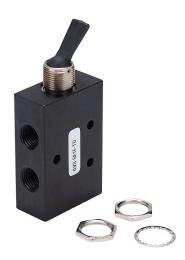
NITRA manual valve, 5-port (4-way), 2-position, toggle style actuator, detented, 1/8in female NPT inlet(s), 1/8in female NPT outlet(s), 1/8in female NPT exhaust(s), Cv=0.37, through panel mount.
