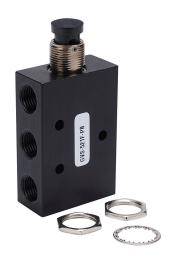
NITRA pneumatic manual valve, 5-port (4-way), 2-position, pushbutton, spring return, 1/8in female NPT inlet(s), 1/8in female NPT outlet(s), 1/8in female NPT exhaust(s), Cv=0.37, through panel mount.
