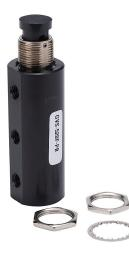
NITRA pneumatic manual valve, 5-port (4-way), 2-position, pushbutton, spring return, #10-32 female UNF inlet(s), #10-32 female UNF outlet(s), #10-32 female threaded exhaust(s), Cv=0.23, through panel mount.
