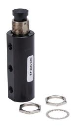
NITRA manual valve, 5-port (4-way), 2-position, pushbutton, spring return, #10-32 female threaded inlet(s), #10-32 female threaded outlet(s), #10-32 female threaded exhaust(s), Cv=0.23, through panel mount.
