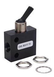
NITRA manual valve, 3-port (3-way), 2-position, N.C., toggle style actuator, detented, side ports, 1/8in female NPT inlet(s), 1/8in female NPT outlet(s), 1/8in female NPT exhaust(s), Cv=0.42, through panel mount.
