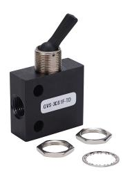
NITRA pneumatic manual valve, 3-port (3-way), 2-position, N.C., toggle style actuator, detented, side ports, 1/8in female NPT inlet(s), 1/8in female NPT outlet(s), 1/8in female NPT exhaust(s), Cv=0.42, through panel mount.
