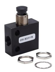
NITRA manual valve, 3-port (3-way), 2-position, N.C., pushbutton, spring return, side ports, 1/8in female NPT inlet(s), 1/8in female NPT outlet(s), 1/8in female NPT exhaust(s), Cv=0.42, through panel mount.
