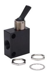
NITRA pneumatic manual valve, 3-port (3-way), 2-position, N.C., toggle style actuator, detented, 1/8in female NPT inlet(s), 1/8in female NPT outlet(s), vent hole exhaust(s), Cv=0.42, through panel mount.
