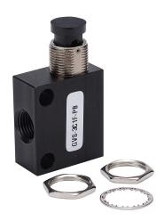
NITRA pneumatic manual valve, 3-port (3-way), 2-position, N.C., pushbutton, spring return, 1/8in female NPT inlet(s), 1/8in female NPT outlet(s), (1) vent hole exhaust(s), Cv=0.42, through panel mount.
