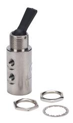
NITRA pneumatic manual valve, 3-port (3-way), 2-position, N.C., toggle style actuator, detented, 90-degree ports, #10-32 female UNF inlet(s), #10-32 female UNF outlet(s), #10-32 female threaded exhaust(s), Cv=0.27, through panel mount.
