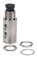
NITRA pneumatic manual valve, 3-port (3-way), 2-position, N.C., pushbutton, spring return, 90-degree ports, #10-32 female UNF inlet(s), #10-32 female UNF outlet(s), #10-32 female threaded exhaust(s), Cv=0.27, through panel mount.
