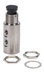
NITRA manual valve, 3-port (3-way), 2-position, N.C., pushbutton, spring return, 90-degree ports, #10-32 female threaded inlet(s), #10-32 female threaded outlet(s), #10-32 female threaded exhaust(s), Cv=0.27, through panel mount.
