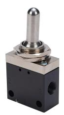
NITRA pneumatic manual valve, 3-port (3-way), 3-position, center exhaust, toggle style actuator, spring return, 1/8in female NPT inlet(s), 1/8in female NPT outlet(s), (1) vent hole exhaust(s), Cv=0.54, through panel mount.
