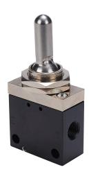
NITRA manual valve, 3-port (3-way), 3-position, center exhaust, toggle style actuator, detented, 1/8in female NPT inlet(s), 1/8in female NPT outlet(s), (1) vent hole exhaust(s), Cv=0.54, through panel mount.
