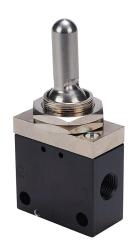
NITRA pneumatic manual valve, 3-port (3-way), 3-position, center exhaust, toggle style actuator, detented, 1/8in female NPT inlet(s), 1/8in female NPT outlet(s), (1) vent hole exhaust(s), Cv=0.54, through panel mount.
