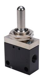
NITRA manual valve, 2-way, 3-position, center closed, toggle style actuator, spring return, 1/8in female NPT inlet(s), 1/8in female NPT outlet(s), Cv=0.54, through panel mount.
