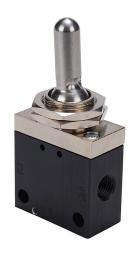
NITRA pneumatic manual valve, 2-way, 3-position, center closed, toggle style actuator, detented, 1/8in female NPT inlet(s), 1/8in female NPT outlet(s), Cv=0.54, through panel mount.
