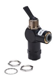
NITRA pneumatic manual valve, 3-port (3-way), 2-position, N.C., toggle style actuator, detented, 90-degree ports, 1/4in push-to-connect inlet(s), 1/4in push-to-connect outlet(s), (1) vent hole exhaust(s), Cv=0.23, through panel mount.
