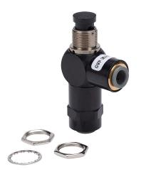
NITRA pneumatic manual valve, 3-port (3-way), 2-position, N.C., pushbutton, spring return, 90-degree ports, 1/4in push-to-connect inlet(s), 1/4in push-to-connect outlet(s), (1) vent hole exhaust(s), Cv=0.29, through panel mount.
