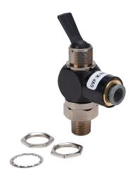
NITRA pneumatic manual valve, 3-port (3-way), 2-position, N.C., toggle style actuator, detented, 90-degree ports, 1/8in male NPT inlet(s), 1/4in push-to-connect outlet(s), (1) vent hole exhaust(s), Cv=0.23, through panel mount.
