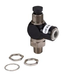
NITRA pneumatic manual valve, 3-port (3-way), 2-position, N.C., pushbutton, spring return, 90-degree ports, 1/8in male NPT inlet(s), 1/4in push-to-connect outlet(s), (1) vent hole exhaust(s), Cv=0.29, through panel mount.
