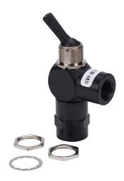
NITRA manual valve, 3-port (3-way), 2-position, N.C., toggle style actuator, detented, 90-degree ports, 1/8in female NPT inlet(s), 1/8in female NPT outlet(s), (1) vent hole exhaust(s), Cv=0.23, through panel mount.
