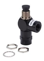
NITRA pneumatic manual valve, 3-port (3-way), 2-position, N.C., pushbutton, spring return, 90-degree ports, 1/8in female NPT inlet(s), 1/8in female NPT outlet(s), (1) vent hole exhaust(s), Cv=0.29, through panel mount.
