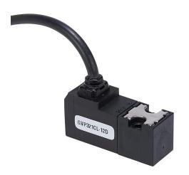
NITRA solenoid valve, 3-way, 2-position, N.C., single latching solenoid spring return, 15mm wide body, Cv=0.047, 12 VDC, 300mm 24AWG pigtail.
