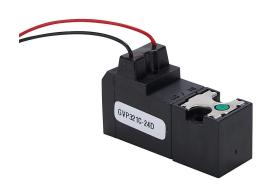
NITRA solenoid valve, 3-way, 2-position, N.C., single solenoid spring return, 15mm wide body, Cv=0.047, 24 VDC, 300mm 24AWG pigtail.
