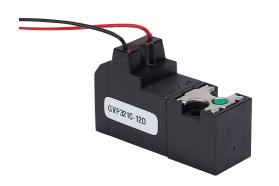
NITRA solenoid valve, 3-way, 2-position, N.C., single solenoid spring return, 15mm wide body, Cv=0.047, 12 VDC, 300mm 24AWG pigtail.
