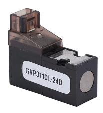
NITRA solenoid valve, 3-way, 2-position, N.C., single latching solenoid spring return, 10mm wide body, Cv=0.013, 24 VDC, miniature pin plug.
