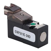
NITRA solenoid valve, 3-way, 2-position, N.C., single solenoid spring return, 10mm wide body, Cv=0.013, 24 VDC, miniature pin plug.
