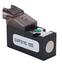
NITRA solenoid valve, 3-way, 2-position, N.C., single solenoid spring return, 10mm wide body, Cv=0.013, 12 VDC, miniature pin plug.
