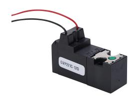
NITRA solenoid valve, 2-way, 2-position, N.C., single solenoid spring return, 15mm wide body, Cv=0.047, 12 VDC, 300mm 24AWG pigtail.
