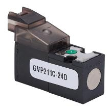
NITRA solenoid valve, 2-way, 2-position, N.C., single solenoid spring return, 10mm wide body, Cv=0.013, 24 VDC, miniature pin plug.
